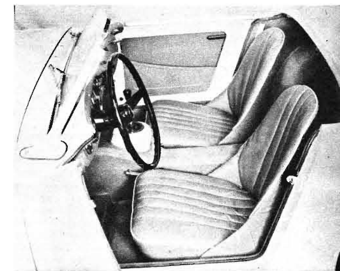
SET alongside the deep propeller-shaft tunnel, the seats have comfortably deep cushions and well-curved squabs to provide lateral support.
