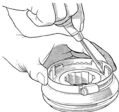
Fig. 13. Pushing down the thrust members.
